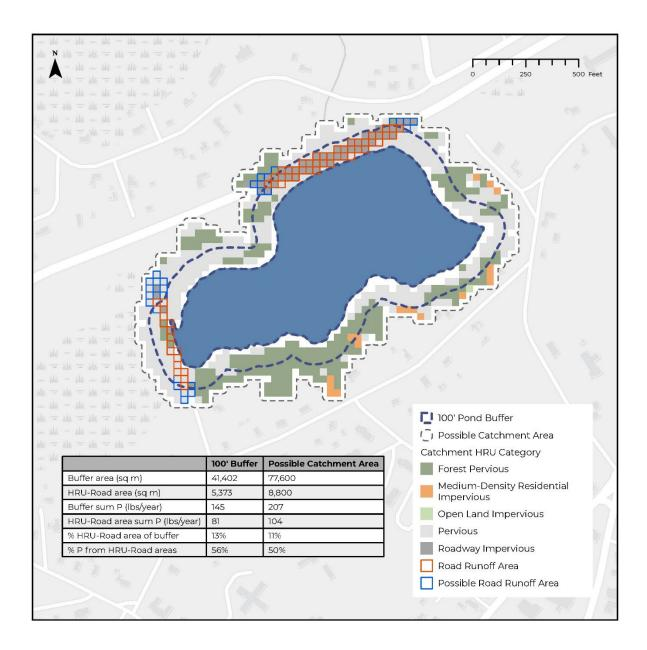
FIGURE 3. Example pond and 100-foot buffer showing HRUs and phosphorus contribution to the pond from roads and other land use acivities.
