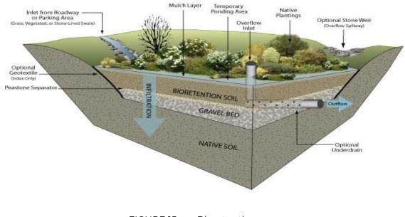
FIGURE 15. Bioretention (Source: Douglas County Environmental Services)
